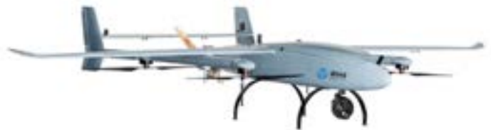
AEROGARD V3900 -H VTOL "AYBARS-2" (Hybrid, Electric + Liquid Fuel Engine, Payload 5 Kg)
