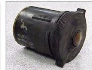
BATTERY COOLANT UNIT (BCU)
